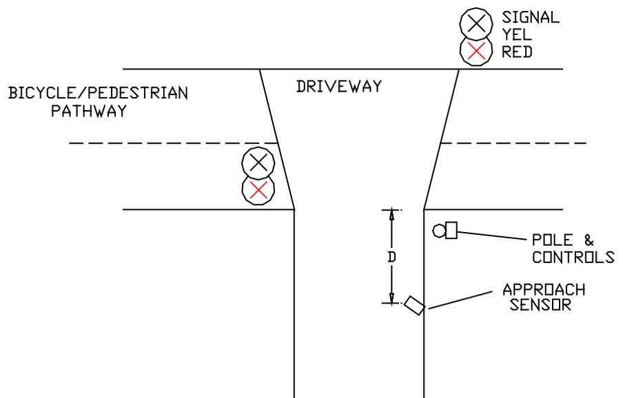
Figure 1: Typical blind driveway application with approach-only sensor
