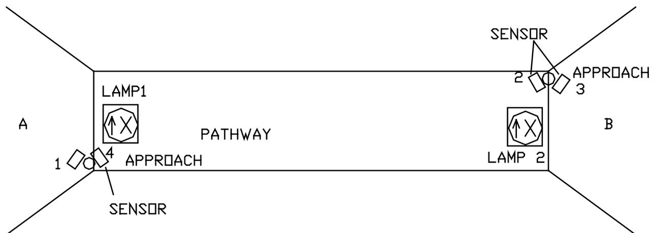
*Figure 1: Typical single lane application with approach only sensors*
