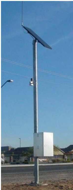
Figure 3, optical detector unit with radio transmitter located to look up the station driveway.
