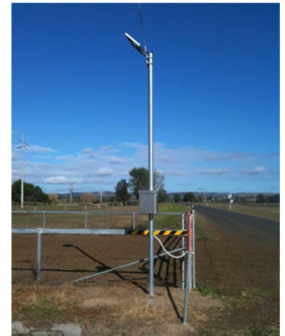
Transmitter system detects when gate is open using a magnetic reed relay.
