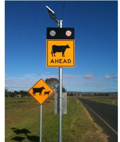
System flasher is used twice daily to move cattle between pastures.
